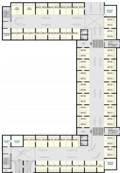
BASEMENT 1 PLAN No. of parking spaces = 79 units
